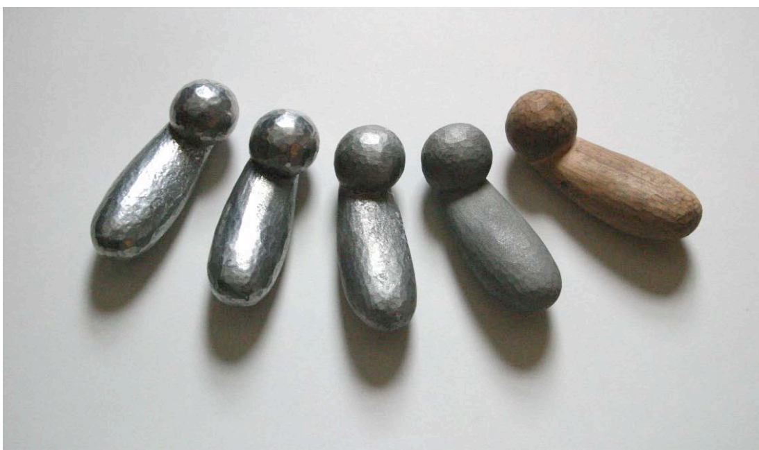
Fig. 17 Wooden pattern and aluminum casts, sculpture made by the author while apprentice to Gretar Mar Thorvaldsson, 2003.
