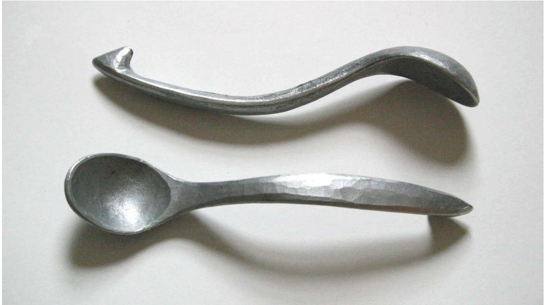
Fig. 16 Cast aluminum spoons, made by the author while apprentice to Gretar Mar Thorvaldsson, 2003.
